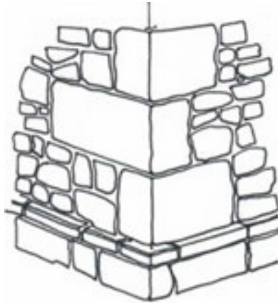
Example of a quoin based on illustration from AngloSaxon Architecture by H M and J Taylor
